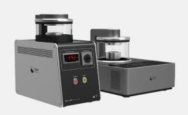
The Ion Sputter Coater allows for imaging of nonconductiv e samples in high vacuum mode for the highest resolutio n imaging. Sputter coaters increase conductivity bycoatin g the test specimen with a few nanometer thick metal film At or Pt. The higher conductivity increases the amount o becondary electron generation and creates higher resolutio n images.
